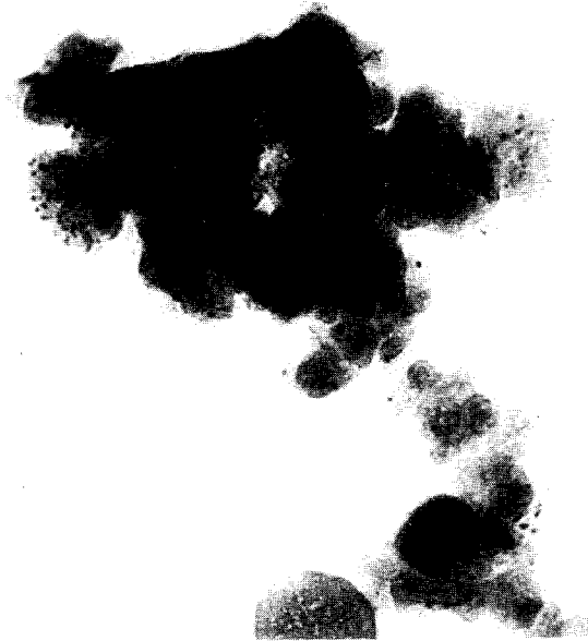
FIG. 11. Transmission electron micrographs of the Pt 1.0% washed sample on B 230 (effective Pt% = 0.31); × 176,000.
